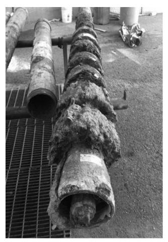
Rusted pumping unit removed from Tremont Street well
