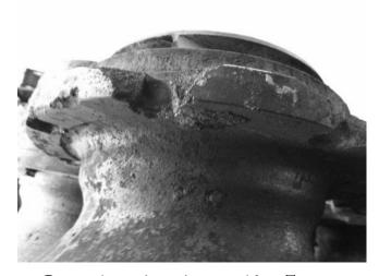
Damaged pumping unit removed from Tremont Street well
