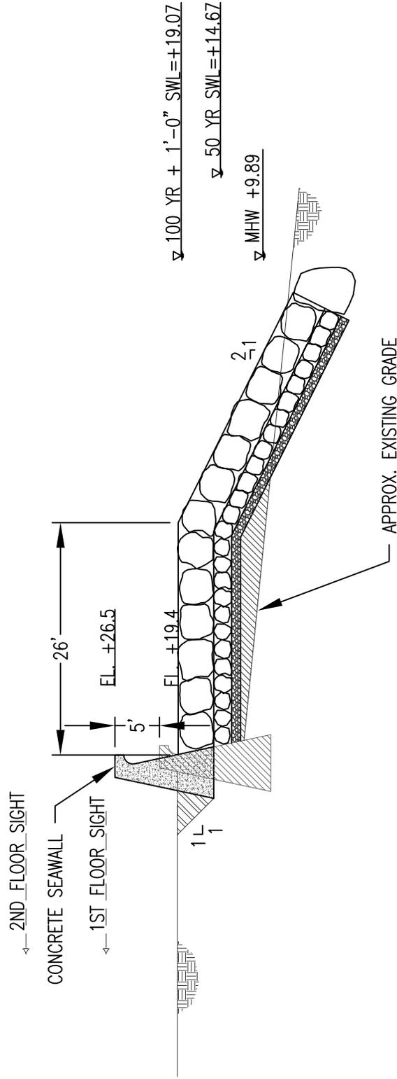
**A** **8** ALTERNATIVE #6 - TOP OF WALL EL. +26.5 & REVETMENT TO EL. +19.4
