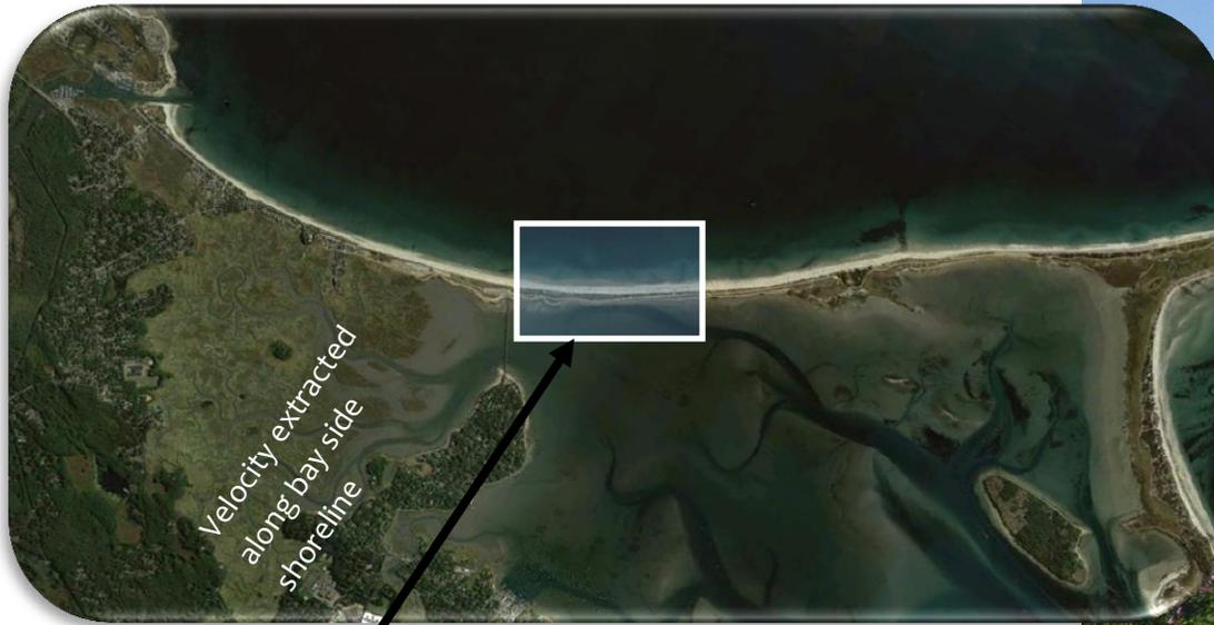
Peak velocities are significantly higher in the channel that runs adjacent to the bayside shoreline. This corresponds to a significant area of ongoing erosion along the bayside shoreline. While swift during even normal tidal conditions as shown here, these velocities approximately double during storm events.
