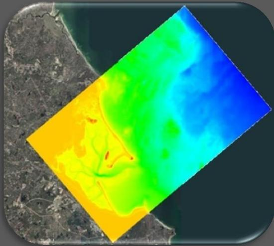
The regional, offshore grid is comprised of 506 cells in the cross-shore direction and 330 cells in the alongshore direction at a resolution of 50 m (165 ft). The offshore boundary of the regional grid is at approximately the 55-meter (180 ft) depth contour.
