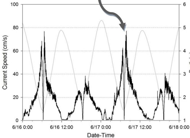
During spring tides, the currents speeds are at a maximum surrounding slack low tide and occur both during ebb and flood flows indicating a shallow water dominant condition. Velocities are much larger during spring tide conditions.
