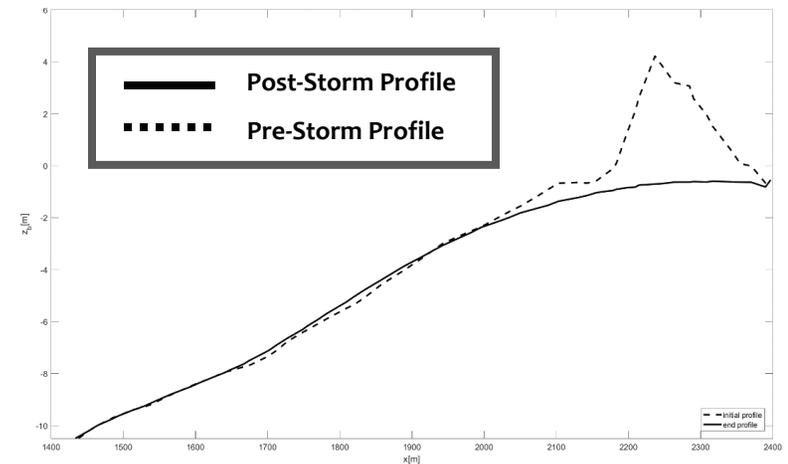
Response of the beach profile (showing cross-shore movement of sediment) fronting the Pavilion region during a 50-year return period storm event. Model results indicate significant erosion of the dune with a majority of the sediment being pushed landward towards and into Duxbury Bay. The dune has been completely eroded.
