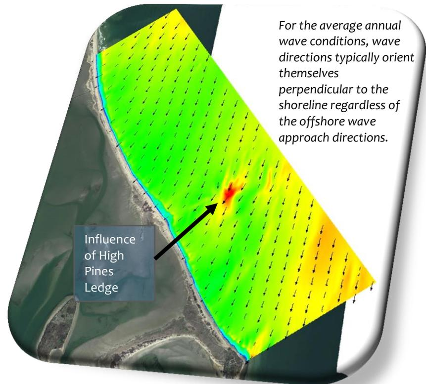
For the average annual wave conditions, wave directions typically orient themselves perpendicular to the shoreline regardless of the offshore wave approach directions.
