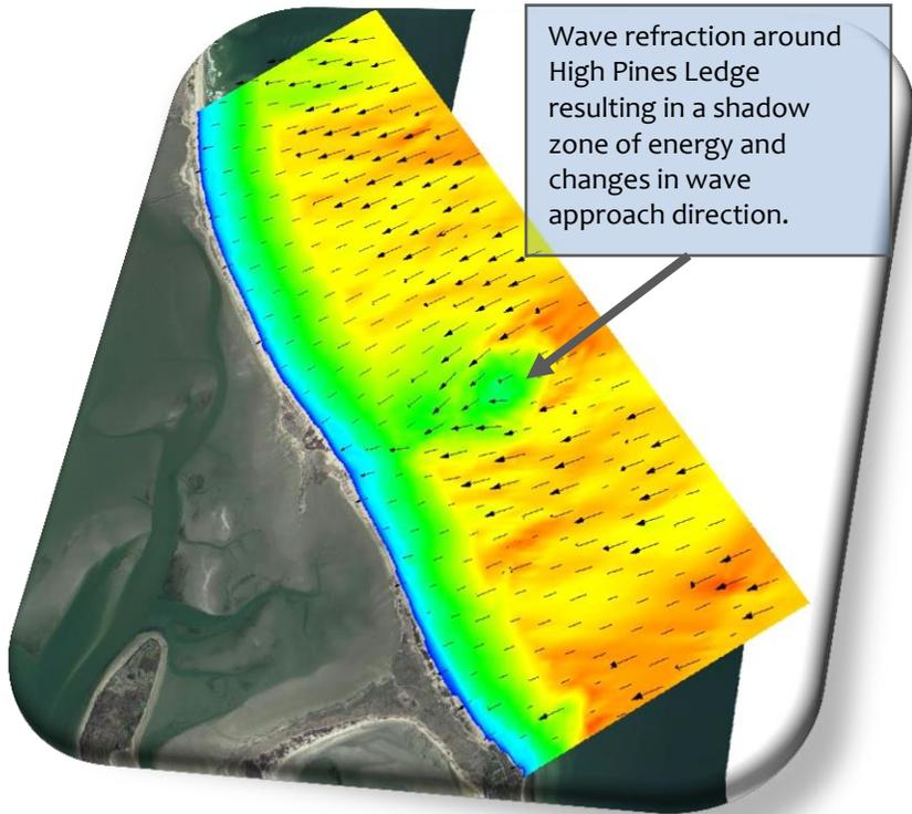
Wave refraction around High Pines Ledge resulting in a shadow zone of energy and changes in wave approach direction.
