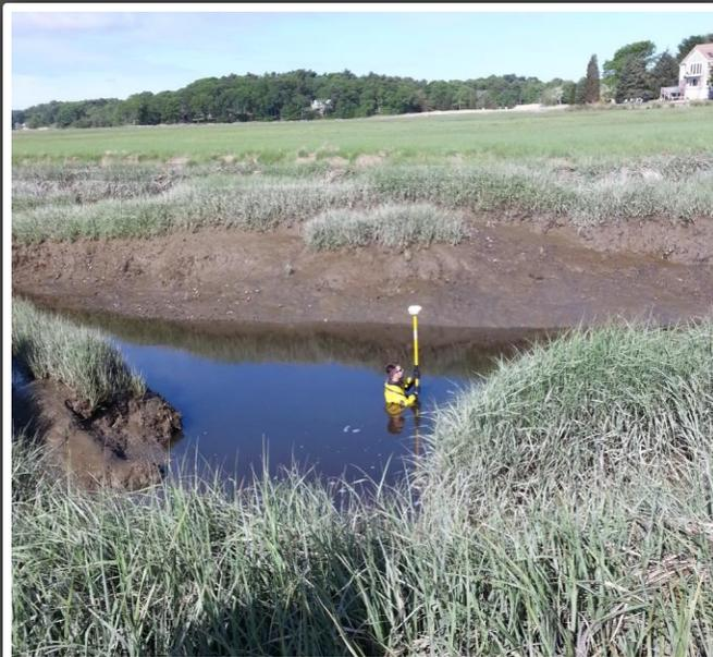
Location of tide gauge in the Upper Marsh of Duxbury Bay. All gauges were surveyed into a vertical datum (North American Vertical Datum of 1988) using an RTK-GPS system.
