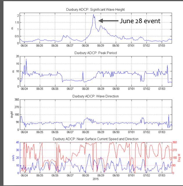
Generally, wave energy was minimal during the deployment period, coinciding with summer conditions. However, a couple of time periods during the deployment had increased wave energy (June 1 and June 28, 2015). These two events were important for testing the accuracy of the wave model. Further discussion on the wave data and model application can be found in Appendix 5-A.
