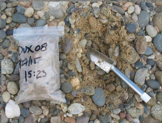
Beach sediment sample taken at station 8 along Duxbury Beach. This sample was located on the bay side of the barrier beach and consisted of a sand and gravel mix. The median grain size was 1.6 mm.
