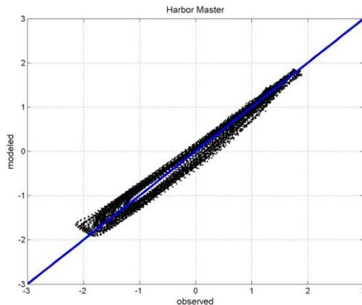
Statistical results of water surface elevations calibration.
