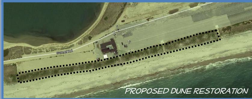
The current state of the dunes in front of the Pavilion is less than ideal. The dunes have narrowed to 20-25 feet in width and are sparsely vegetated. The proposed adaptation consists of a dune and beach berm restoration project spanning approximately 1,000 feet of shoreline. The restoration proposes to restore the dune to a similar level as the adjacent healthy dunes while adding a fronting beach berm.
