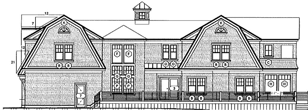
④ SOUTH ELEVATION WINDOW 1/8" = 1'-0"
