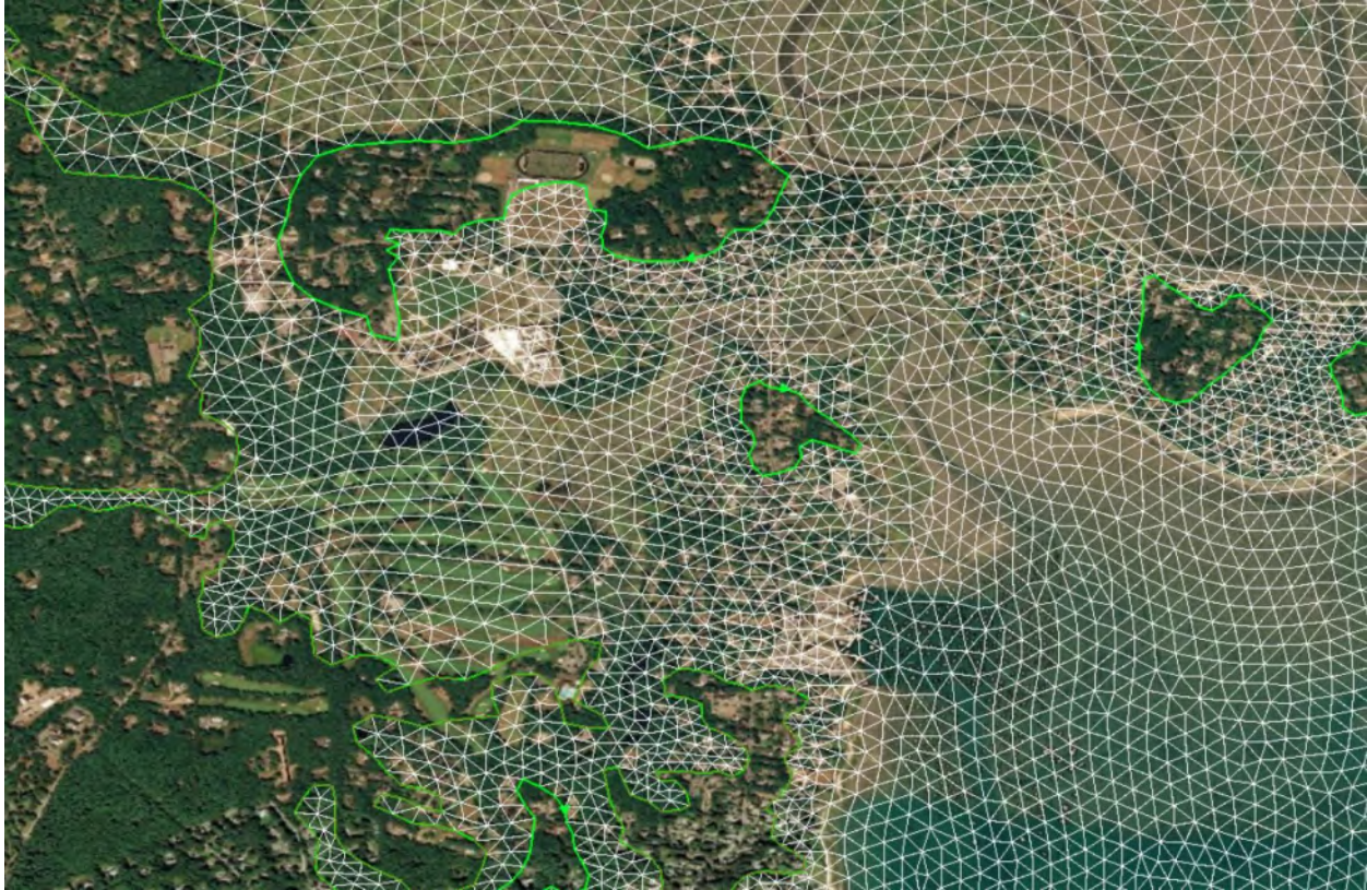
Figure 2-1 Massachusetts Coast Flood Risk Model mesh in Duxbury study area
