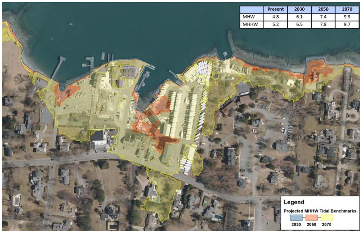
Figure 2-2 Projected Nuisance Flooding (MHHW elevation in feet NAVD88) for Snug Harbor
